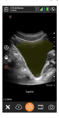
It is necessary to capture both sagittal and transverse images. To display the length, width, and height of the bladder, pause the acquisition by pressing the **Freeze** button. The calipers will be placed automatically depending on the view, with measurements
