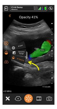
**6.** The opacity of the mask can be varied by dragging the slider control horizontally. Dragging it to the left will reduce the opacity of the segmentation mask while dragging it to the right will increase the opacity of the mask.
