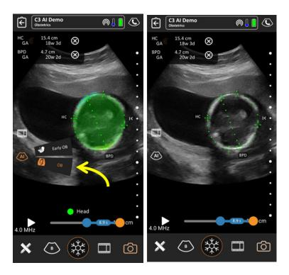
**8.** Manually adjust measurements: To adjust the measurements manually, freeze the image by pressing the **Freeze** button. Then adjust the measurement by dragging the caliper crosshairs.
