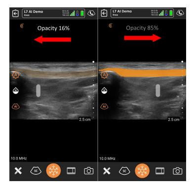
Manually adjust measurements: To adjust the measurements manually, freeze the image by pressing the Freeze button. Then remove the AI predicted overlay mask from the image by pressing the AI button. After disabling the AI feature, only the measurement calipers will remain on the image as shown in the figure below. Adjust the measurement by moving the caliper crosshairs.
