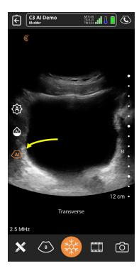
**5.** Once activated, and the bladder is in view, the bladder is automatically highlighted by a yellow mask on top. The highlighted bladder is shown in the picture below.
