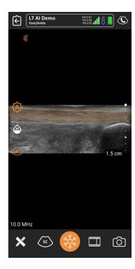
**5.** Once a tendon is detected and highlighted by an orange mask, the tendon thickness can be calculated. To display the tendon thickness, pause the acquisition by pressing on the Freeze button. The calipers will be placed automatically, and the tendon thickness will be displayed in the top left corner of the screen.
