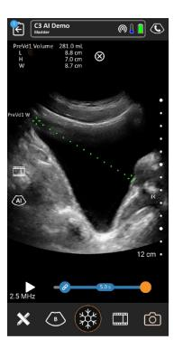
**7.** The opacity of the mask can also be adjusted by making sure the Slider Control carousel wheel is selected to be on "Al Opacity". Scroll directions are highlighted by the red arrow in the images below. Opacity is displayed upon change.
