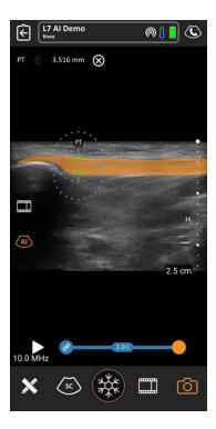
To remove the segmentation mask and disable the AI, tap the AI button until it turns white. As a reminder, AI button color orange signifies-> ON, whereas white signifies-> OFF. The tendon mask can also be disabled in Freeze mode. Once the acquisition is Frozen, disable the AI by tapping the button (color should change from orange -> white). This is particularly useful for users who want to see the tendon thickness without the tendon mask overlay. Refer to the image below.
