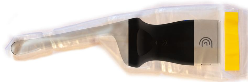
When you have finished using the Clarius Scanner EC7 HD, immediately clean it (for instructions see *Cleaning the Clarius Scanner HD* on page 41), followed by another high-level disinfection. If a Clarius Fan HD (CIDN 50-02-00061) was used, remove the fan prior to the high-level disinfection and follow the instructions for an intermediate-level disinfection (for instructions see *Disinfecting the Clarius Fan HD* on page 44).
